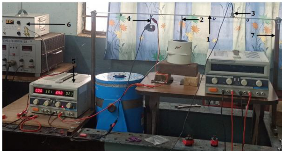
Fig. 1. Photograph showing position of accelerometer and Exciter.1. Aluminum Fixed Beam 2. Stylus of Exciter 3. Accelerometer 4. SMA Spring DVA 5. Dual Mode Power supply 6. Function Generator 7. Fixture for mounting the Beam.
