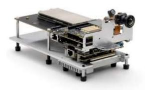
processing capabilities on the RB6 are available through its enhanced Qualcomm AI Engine, which is capable of 70 to 200 trillion operations per second (TOPS). Aside from the hardware, the Qualcomm Robotics RB6 platform includes an integrated, premium AI software development kit (SDK): the Qualcomm Intelligent Multimedia SDK. The SDK blends "multimedia, AI and ML, computer vision, and networking building blocks to support the end-to-end deployment of robotic applications," states Qualcomm.
