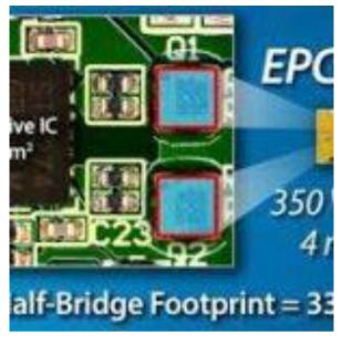
The EPC2050 measures just 1.95 mm x 1.95 mm. This tiny size enables power solutions that occupy ten times less area than comparable silicon solutions.
