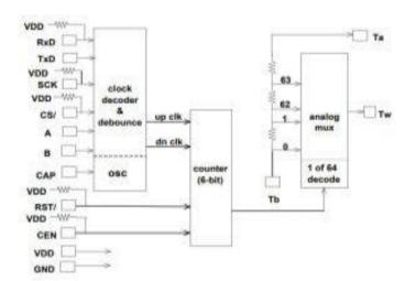
Debounce circuits included where are electromechanical switches are expected, although pull-up resistors must added. "The LSI/CSI digital potentiometers are used as replacements for mechanical potentiometers and for potentiometer adjustments," according to distributor Omni Pro, which will be stocking the parts. "They can also be used for remote adjustments of instrumentation for gain, offset, time constant, line impedance matching or audio equipment volume control."
