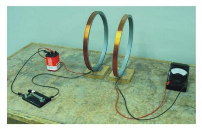
Inductive charging (also known as "wireless charging") uses an electromagnetic field to transfer energy between two objects. This is usually done with a charging station. Energy is sent through an inductive coupling to an electrical device, which can then use that energy to charge batteries or run the device.
